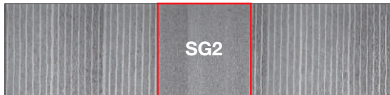
Under microscope at 100x magnification The core material is SG2 and is covered by 50 layers on each side.
